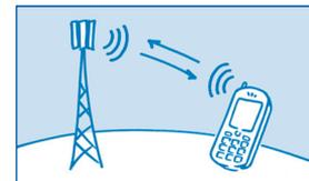
So every mobile radio station knows which mobile phones are turned on within its range. This area which provides every mobile radio station with reception is also called a **radio cell**.
