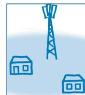
The individual radio stations are connected with a central **radio switching station** via point-to-point radio or cable. This central switching computer knows the locations of all mobile phones that are turned on and forwards data from one radio cell to another and also to a different telephone network.
